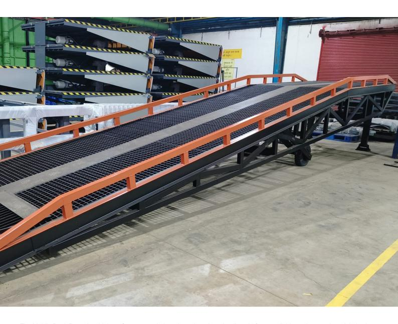
The Mobile Dock Ramp is a high-performance solution where there is no loading platform available on the premises. It helps in rapid loading and unloading of goods; forklifts and handling trucks can directly travel over this too quickly to load or unload goods, and the working efficiency is greatly increased. The set-up of Mobile Dock Ramp can be done anywhere in the ground and provide an ideal solution to bridge the difference in height between the truck bed and the floor-level area.
